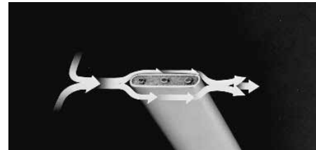
Air Flow Normal to Sheath Geometry
