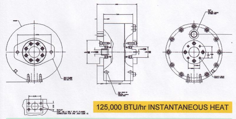
The ISLAND CITY Dynamic-Heat-Generator is a MECHANICALLY DRIVEN fluid heater. Only rotary shaft input is required to heat large fluid volumes rapidly and efficiently without a heat exchanger. ORIGINALLY developed to heat and maintain diesel engine temperature in arctic conditions the DHG is adaptable to many heating applications. Driven from engine PTO, electric motor, hydraulic drive or belt the DHG has one moving functional component requiring no regular service or consumables.
