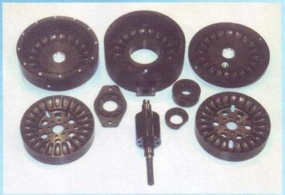
Simple and rugged characterizes the Island City DHG construction.. Monolithic CNC machined components are TYPE III anodized per MILSPEC for corrosion and erosion protect. Hard housing surface finish (85 Rockwell) is approved for potable water and food applications. Operating temperature range to 250 deg F [121 deg C] with higher operating temperature available upon application.
