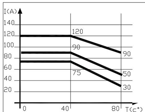
N.B.: Curves for the GTS 120 refer to the device complete with standard running.
