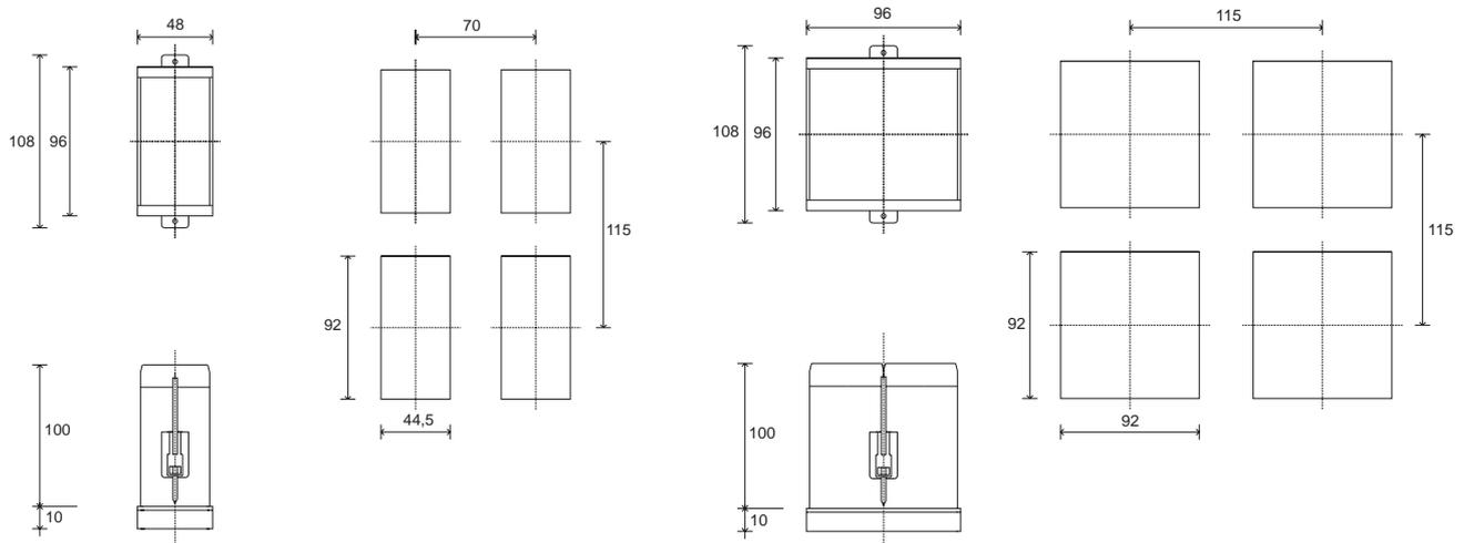
Dimensions: 48x96mm - 96x96mm (1/8DIN - 1/4DIN) depth 100mm
